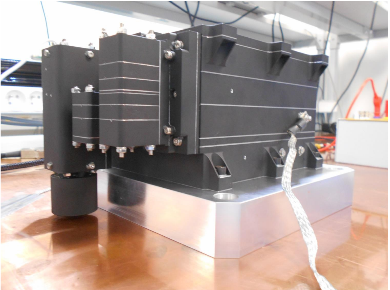
Figure 1 : The ICARE-NG 2 flight model for HotBird-13f with the sensors on the left of the instrument and the electronic box on the the right.
