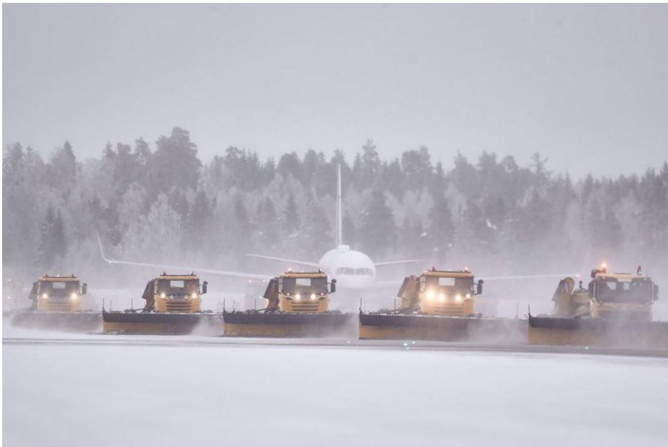
Figure 12: Yeti Move utilizes NMA's RTK-service to ensure precise positioning of the autonomous sweepers. The vehicles shall operate without driver interference on Oslo Airport Gardermoen (OSL), except for an operator located in the first machine. Without the aid of GNSS correction signals, both safety and operational performance would be reduced (Photo: Yeti Move).
