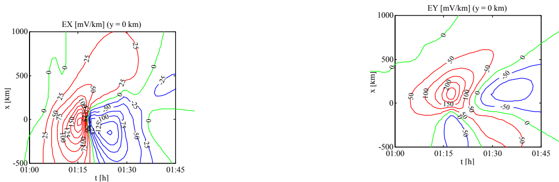
Fig. 5. North component E_x (upper panel) and east component E_y (lower panel) of the electric field at the earth's surface at y = 0 as a function of time starting at 01 h 00 m and at different values of x when the WTS current pattern shown in Fig. 4 moves at a westward velocity of 1 km/s across the area.
