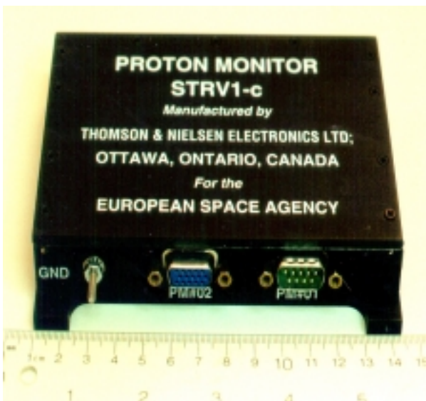
Figure 2 The PM Proto-Flight Model intended for flight on the STRV1-c spacecraft.
