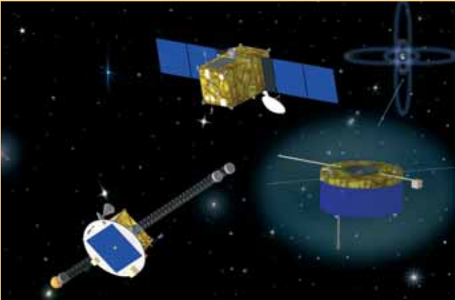
Elements of the space weather system studied within the Concurrent Design Facility (CDF) at ESTEC. This proposed space segment consisted of a solar monitor, a solar wind monitor and a fleet of four inner magnetospheric monitoring spacecraft. Both the solar and solar wind monitors would be permanently situated in the solar wind, in a halo orbit around the L1 Lagrangian point between the Sun and the Earth. The magnetospheric monitors would be located in a series of elliptical orbits within the magnetosphere, taking them through the Earth's radiation belts
