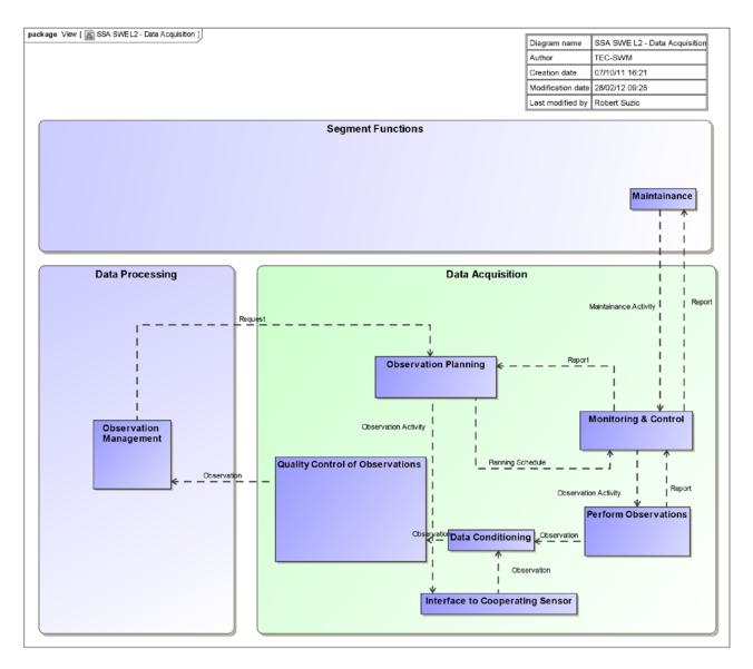
Figure 6: SWE Data Processing Functions
