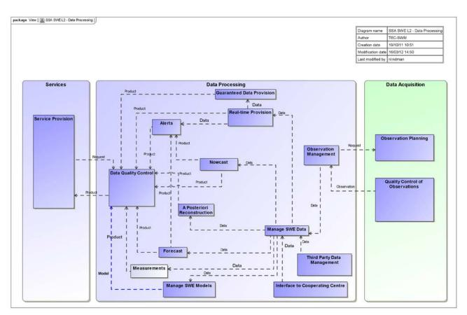
Figure 3: SWE Data Processing Functions
