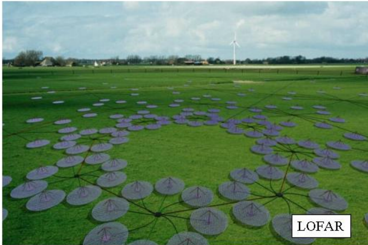
Figure 24. Array of antennas suggested for LOFAR/LOIS.
