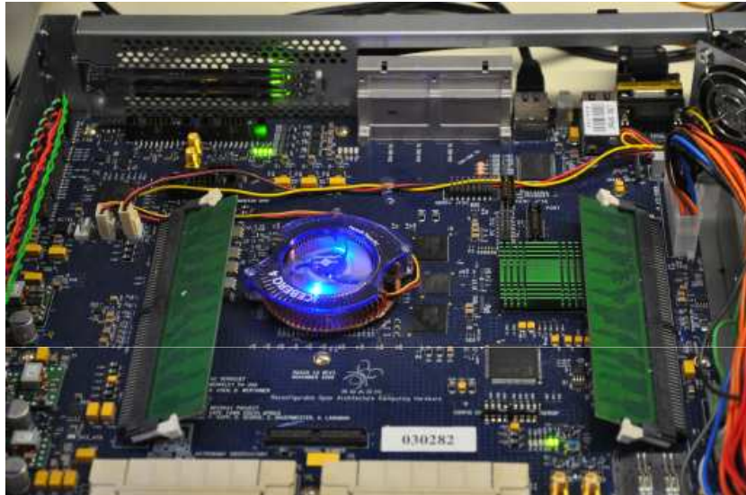
Spectro numérique ROACH 14 bits, 2*500 Msamples/s
